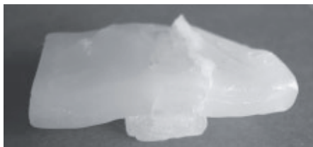
Figure 5: Seesaw wax model after releasing the structures by dissolving the soap.
