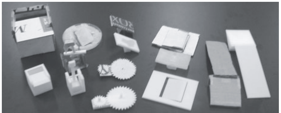
Figure 3: Group picture of all ABS plastic, paper, and wax models. The students chose to model two of the designs using the soap and wax process – the seesaw seen in the center of the drawing and the door shown in the center right.
