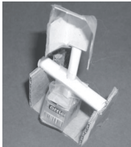
Figure 1: One group of students designed a trebuchet that threw skittles. This is their paper model. The counterweight contains pebbles and playground sand. This model did work, and students were able to shoot Skittles candy into their mouths.
