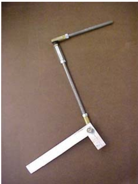
Figure 8. Photograph of the front leg subassembly [2]
