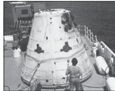
Figure 4: The Frustrum of the SRB is loaded on to the ship
