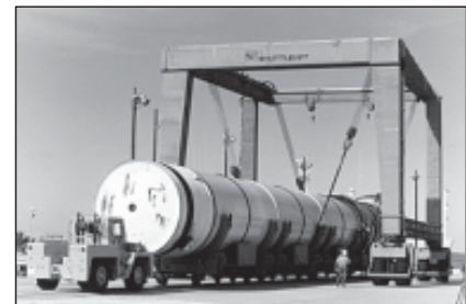
Figure 6: The spent SRB is loaded on to the ship to be transported back to the manufacturer
