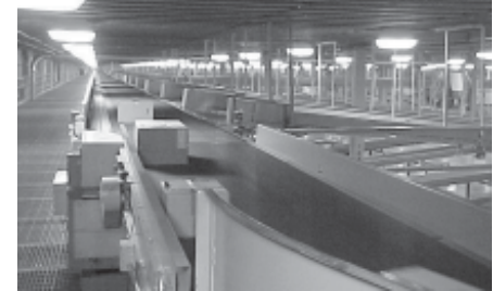
Photograph 6. Carton spacing on the sorter
