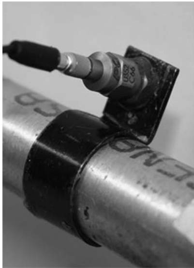
Fig. 11 Accelerometer bracket used for torsional vibration measurement
