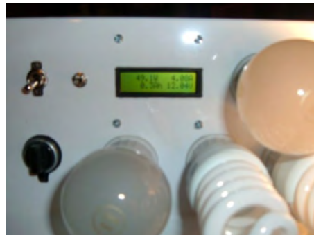
Figure 3. Load display panels that help teachers and students read and record voltage, current, power, and energy values.
