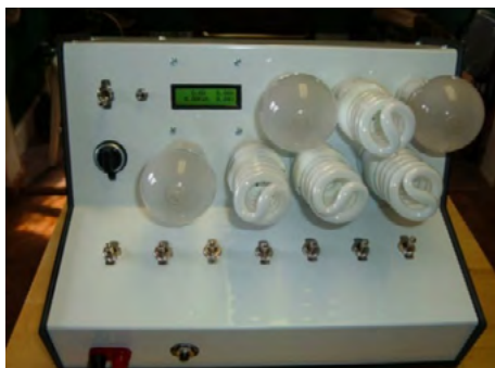
Figure 3. Load display panels that help teachers and students read and record voltage, current, power, and energy values.
