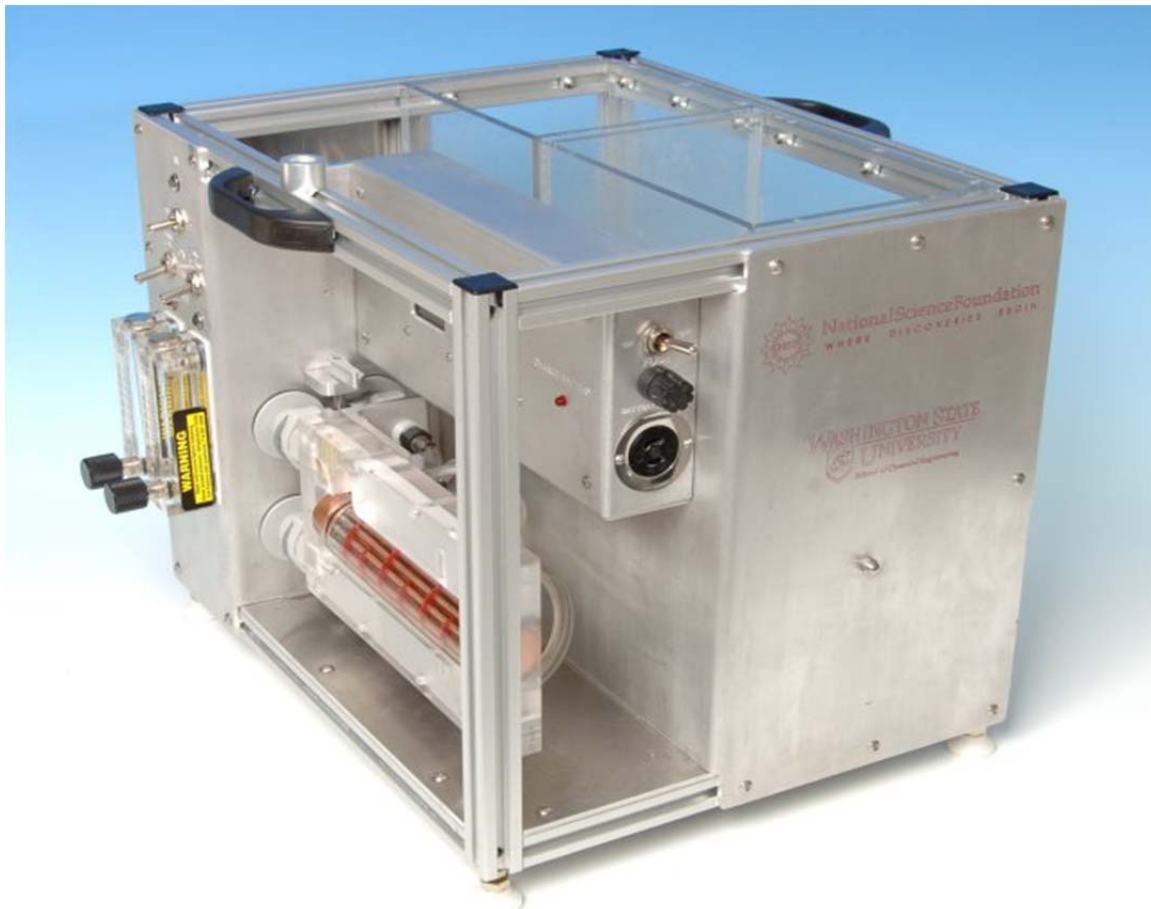
Figure 1. Second generation Desktop Learning Module (DLM) with inserted shell and tube heat exchanger cartridge
