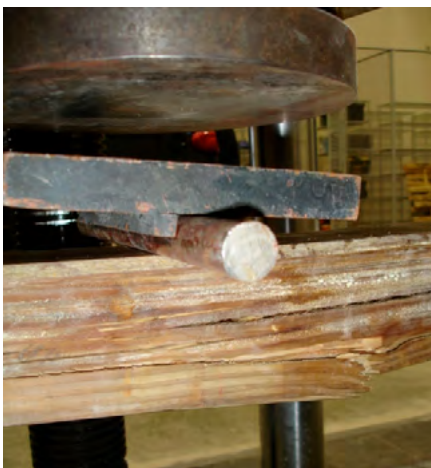
Figure 8: Failure of 4x4 wood member in beam deflection test
