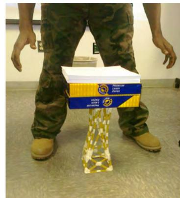
Figure 1. A. A tower supporting a load of 5.7 kg.
