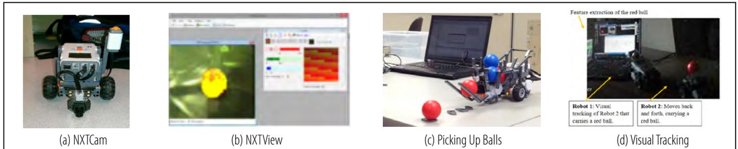
Figure 3. Vision-based control implemented on LEGO NXT.
