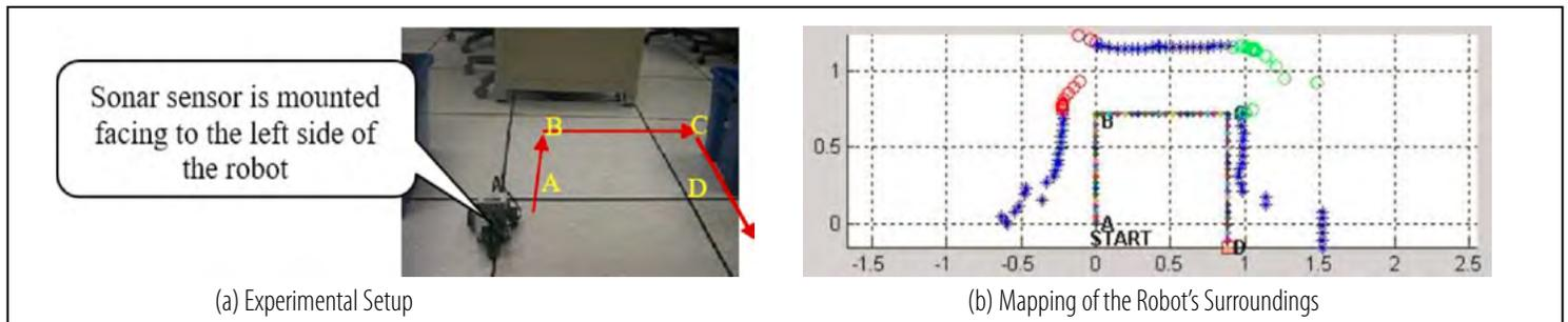
Figure 2. Map building using a sonar range sensor.
